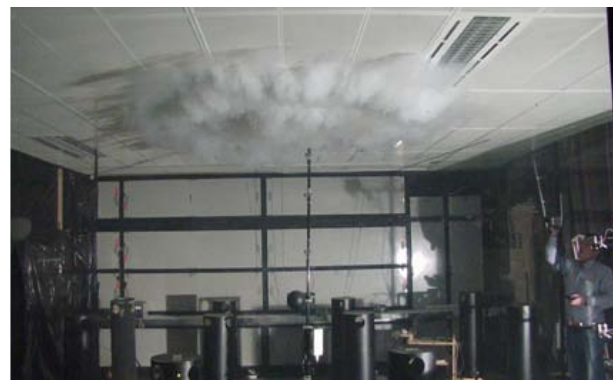
Figure 2: Air flow pattern made visible by smoke tracer
