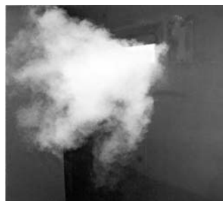
Jet pattern made visible with smoke tracer
